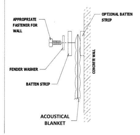
FOR ADDITIONAL SUPPORT, BATTEN STRIPS CAN BE USED AROUND THE PERIMETER OF THE PANEL (AND ACROSS THE PANEL FOR VERY LONG PANELS)
