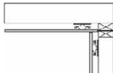
Install ceiling drywall before walls to allow for a fire stop by butting ceiling drywall to studs
