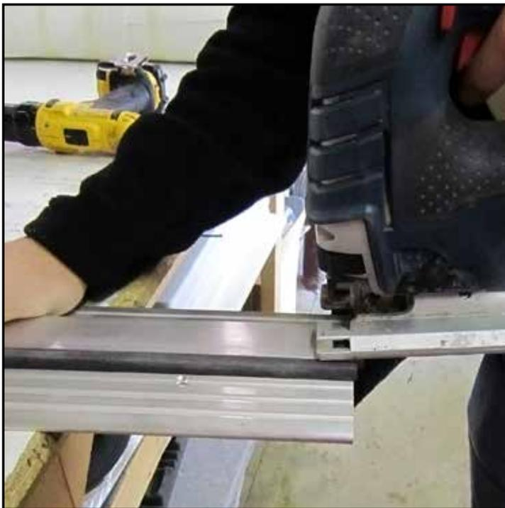
MEASURE, NOTCH & CUT THRESHOLD
