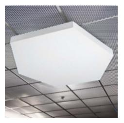
Four points are usually all that is necessary to suspend 4'x4' ceiling clouds in place. Keep corkscrews, hanger wires and anchors overtop in exact alignment, true and plumb. To find the approximate distances away from the sides to install the corkscrew hangers, multiply the width and length by 0.20.
