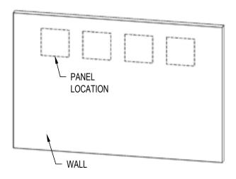
2. SECURE MICORE NAIL CLIPS TO WALL USING APPROPRIATE FASTENERS. CLIPS SHOULD BE LOCATED TO ENSURE THERE IS NO CONTACT BETWEEN CLIPS & FABRIC.
