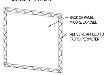
4. ENSURE PANEL IS LOCATED PROPERLY, PRESS PANEL FIRMLY TO WALL. (MAKE SURE THE MICORE CORE IS BEING IMPALED BY THE NAIL CLIPS, NOT THE FABRIC.)
