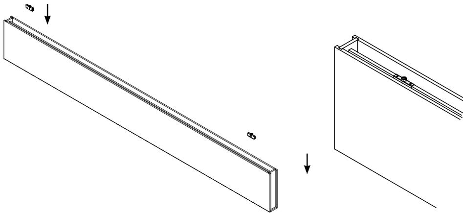
2. Install the threaded rod into the spike bracket.
