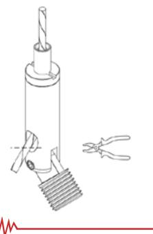
5. Press and hold the spring portion to insert the cable.
