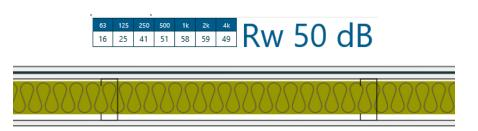
2.3 2x Drywall – Green Glue – RSIC – Studs – MLV – 1x Drywall [with insulation]
