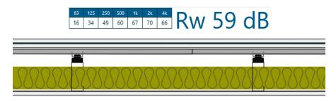
2.4 2x Drywall – Green Glue – RSIC – Studs – MLV – 1x Drywall [w/o insulation]
